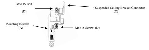
3. Insert chains (not included) through the loop holes of the **Suspended Ceiling Bracket Connector**(C).
