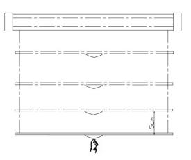
Attention: If the screen does not unlock, carefully pull the screen straight down with a little force. Always pull the screen down at a 90-degree angle.
