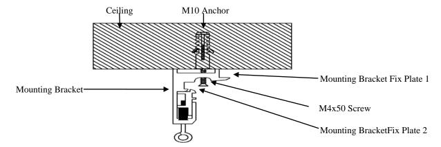
3. Attach the screen to the **Mounting Bracket** (**A**) by inserting the top of the case to **FixPlate 1** and securing the back of the case to **Fix Plate 2**. Make sure the case slots are securely attached to the **Mounting Bracket** (**A**).
